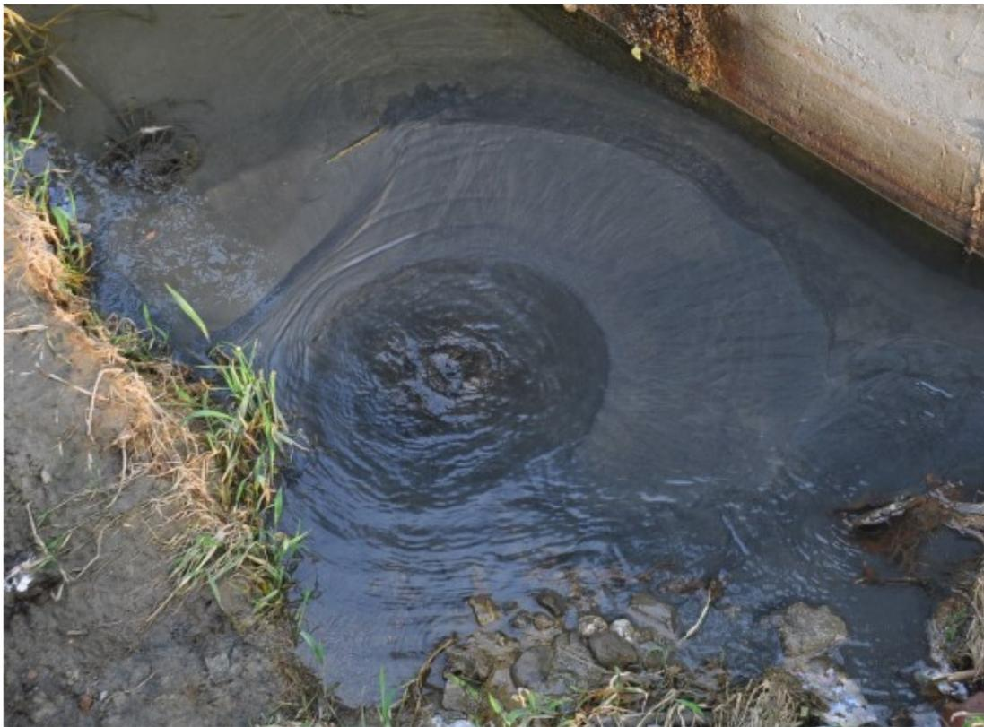
Figure 13. The outflow of silt occurred in the early stage of piping failure (Hsu, 2018).
