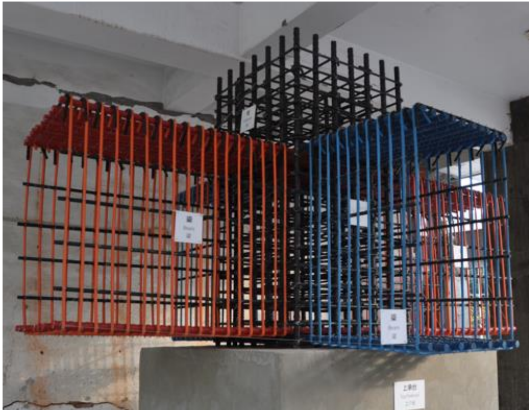
Figure 17. Excessive cross-sectional area and excessive steel reinforcement resulting from revised seismic design code after the 921 Jiji earthquake.
