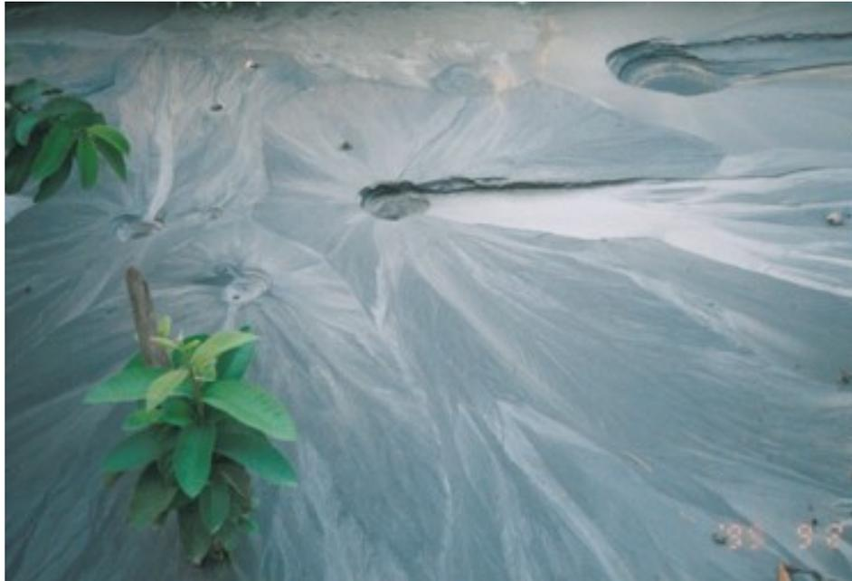
Figure 1. Tubular liquefaction that took place during the Jiji earthquake.
