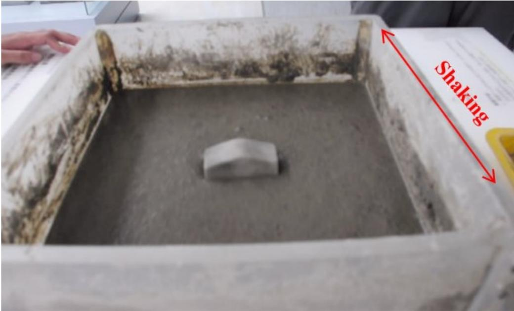
Figure 8. Punching shear failure test of a building model conducted by traditional scholars through a simulation test of the saturated loose sand layer by means of a shaking table (Tsao, 2019).
